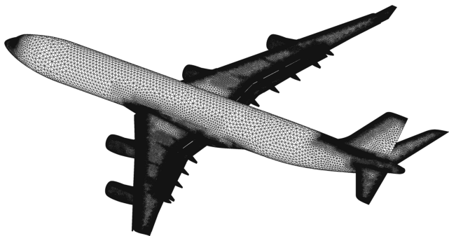
Fig. 7 CFD surface mesh, FULL configuration.
